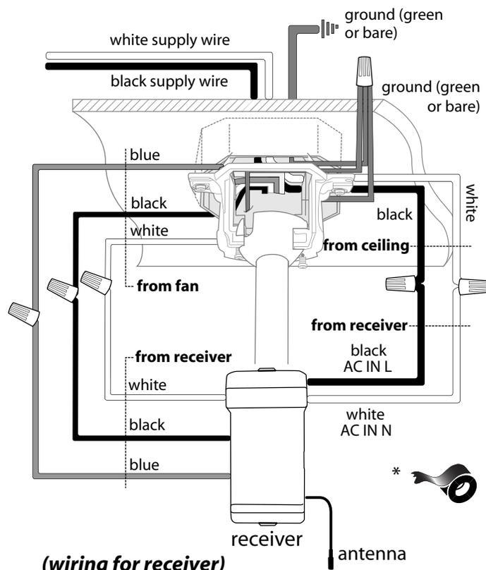
\* Wrap each wire connector separately with electrical tape as an extra safety measure.
